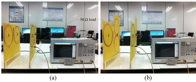
Fig. 9. Experimental setup using network analyzer for signal gain measurement of (a) conventional circular loop antenna array MIMO and (b) heterogeneous multipole loop antenna array MIMO.
